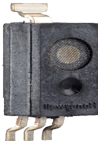
Figure 4: Moisture sensor HIH-5030-001
